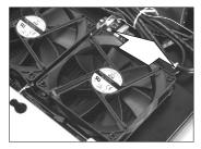
Slide the anti-vibration fan upwards to remove.
