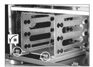
Release the HDD cages by loosening the 2 screws.
