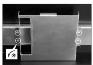
Unscrew the fastening screws to release the slim ODD tray.
