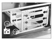
Release the HDD cages by loosening the 2 screws.
