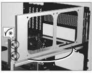
Remove 2 thumb screws to release.
