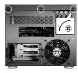
Remove 3 screws to release the top cover.
