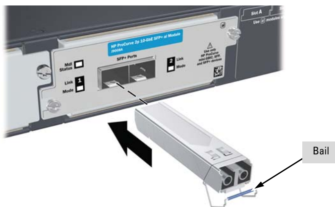
Figure 2-11. Installing a transceiver
