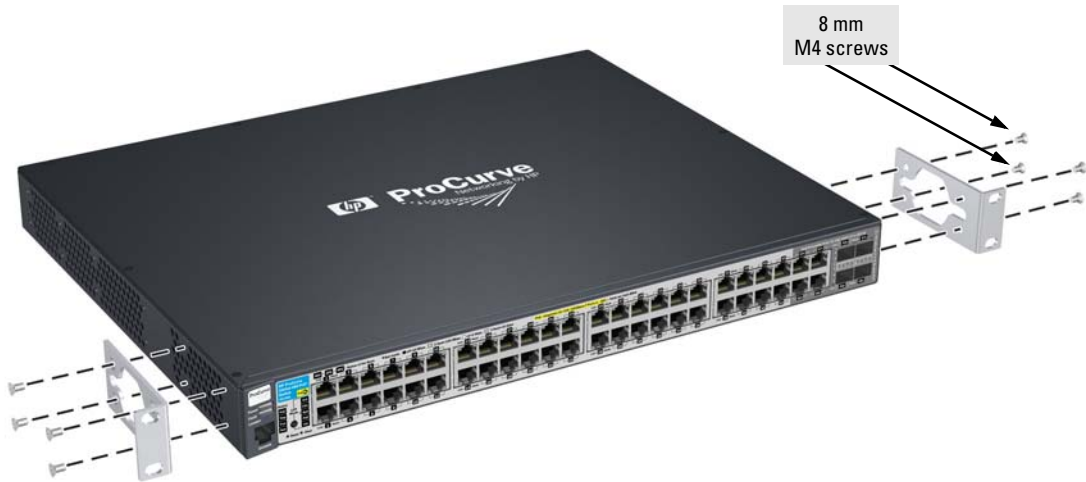
Figure 2-9. Attaching mounting brackets
